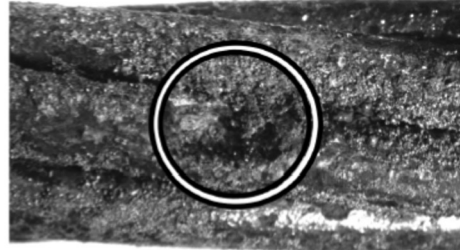
Fig. 11—Example of medium-size pit (sample 39AB); image is 12.6 mm (0.5 in.) wide and 9.5 mm (0.375 in.) high.
