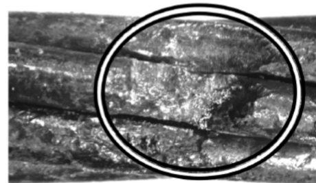
Fig. 12—Example of large-size pit (sample 38CD); image is 12.6mm (0.5 in.) wide and 9.5 mm (0.375 in.) high.
