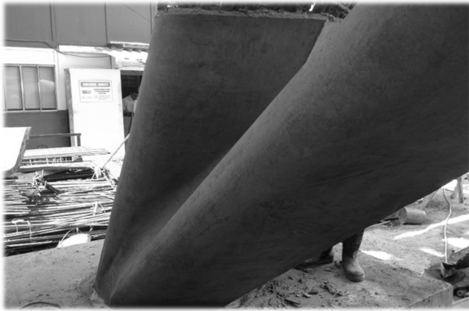
Prototype column: SCC, 50MPa, not vibrated
