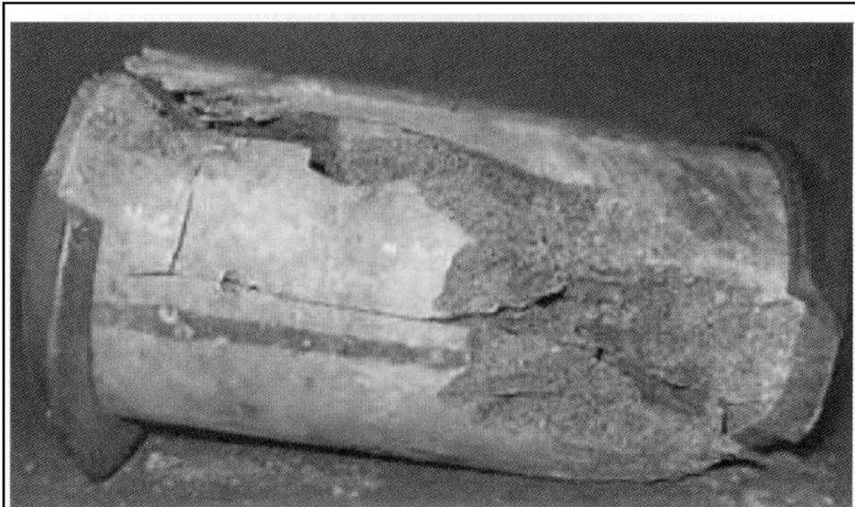
**A compression test specimen. Is this failure mode acceptable? Is there evidence of preparation errors that would impact the test result? A certified CQTM is expected to know the answers**
