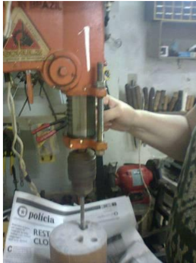
Figure 4. Drilling tests with fixed drill.
