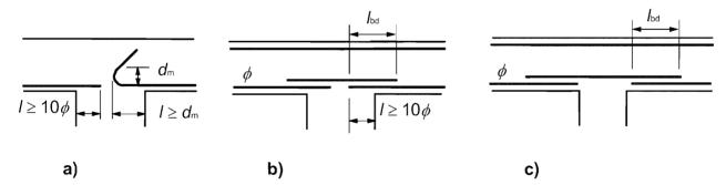
Figure 9.4: Anchorage at intermediate supports
