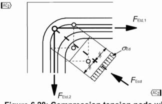
Figure 6.28: Compression tension node with reinforcement provided in two directions
