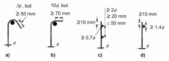
**Note:** For c) and d) the cover should not be less than either  $3\phi$  or 50 mm.
