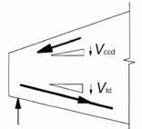
Figure 6.2: Shear component for members with inclined chords
