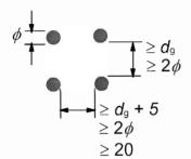
**Note:** Where  $\phi$  is the diameter of pre-tensioned tendon and  $d_q$  is the maximum size of aggregate.
