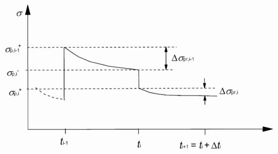
Figure D.1: Equivalent time method
