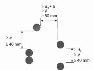
**Note:** Where  $\phi$  is the diameter of post-tension duct and  $d_q$  is the maximum size of aggregate.
