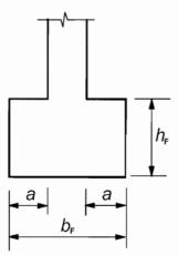
Figure: 12.2: Unreinforced pad footings; notations
