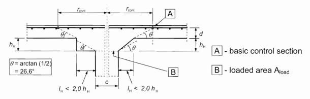
Figure 6.17: Slab with enlarged column head where  $I_{\rm H}$  < 2,0  $h_{\rm H}$
