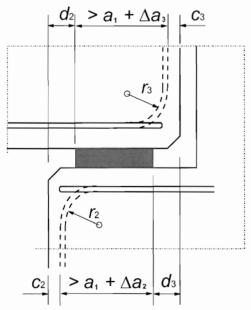
Figure 10.5: Example of detailing of reinforcement in support
