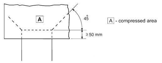
Figure 9.11: Compressed area increasing the anchorage capacity
