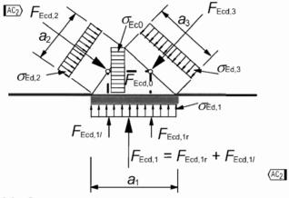
Figure 6.26: Compression node without ties
