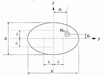
Figure 5.8. Definition of eccentricities e<sub>y</sub> and e<sub>z</sub>.
