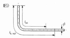
a) Basic tension anchorage length, *l*<sub>b,rqd</sub>, for any shape measured along the centerline (AC1)
