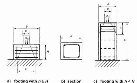
Figure 9.14: Splitting reinforcement in footing on rock
