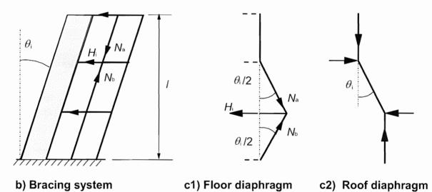
Figure 5.1: Examples of the effect of geometric imperfections
