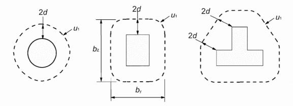
Figure 6.13: Typical basic control perimeters around loaded areas
