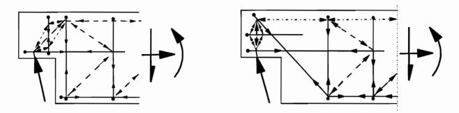
Figure 10.4: Indicative models for reinforcement in half joints.
