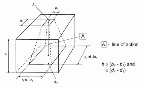
Figure 6.29: Design distribution for partially loaded areas
