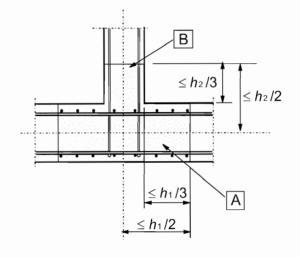
A supporting beam with height  $h_1$  B supported beam with height  $h_2$  ( $h_1 \ge h_2$ )
