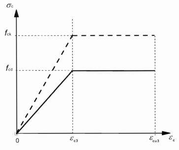
Figure 3.4: Bi-linear stress-strain relation.
