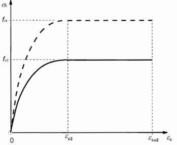
Figure 3.3: Parabola-rectangle diagram for concrete under compression.
