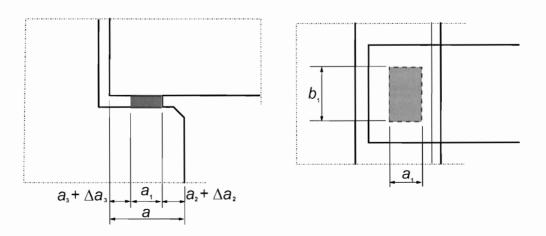
Figure 10.6: Example of bearing with definitions.
