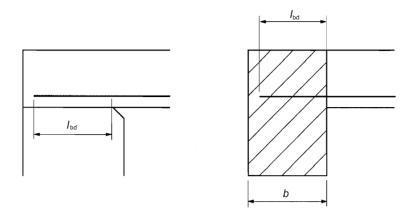
a) Direct support: Beam supported by wall or column
