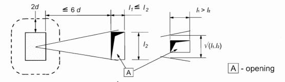
Figure 6.14: Control perimeter near an opening
