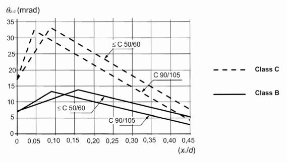
Figure 5.6N: Basic value of allowable rotation,  $\theta_{pl,d}$ , of reinforced concrete sections for Class B and C reinforcement. The values apply for a shear slenderness  $\lambda = 3,0$
