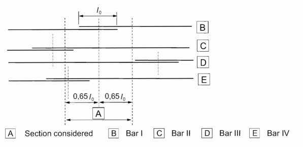
Example: Bars II and III are outside the section being considered: % = 50 and  $\alpha_6 = 1,4$
