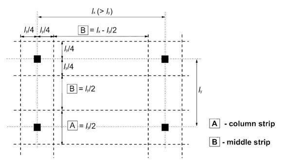
Figure I.1: Division of panels in flat slabs
