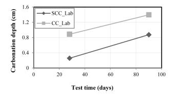
Figure 8. Accelerated carbonation test results.
