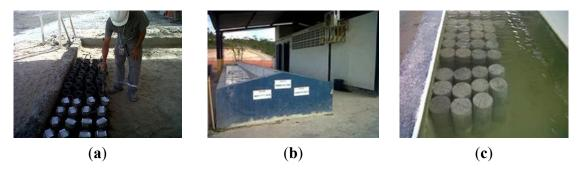
Figure 2. Cure of the samples at laboratory conditions. (a) specimen's casting; (b) curing tank; (c) specimens immersed in the curing tank.
