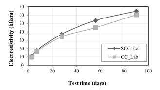
Figure 7. Electrical resistivity test results.
