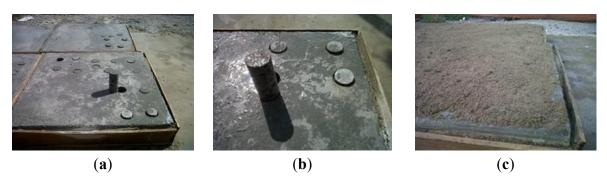
Figure 3. Cure of the specimens at local atmospheric conditions. (a) concrete core; (b) detail of concrete core; (c) concrete block.
