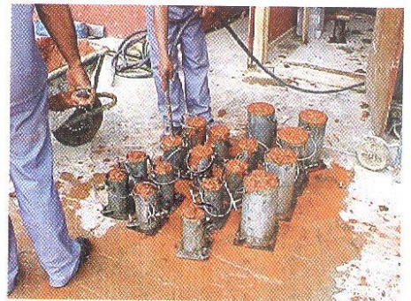
Fig. 6: Test cylinders, 100 x 200 mm and 150 x 300 mm, being prepared at the site
