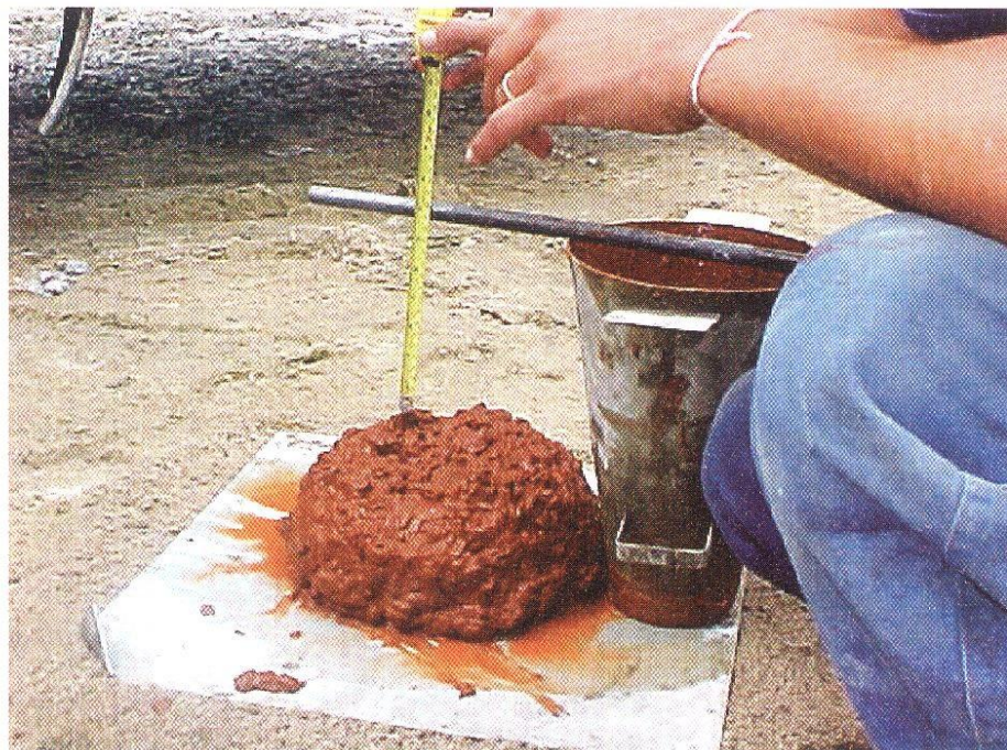
Fig. 4: A slump between 140 and 200 mm proved acceptable for workable HPCC
