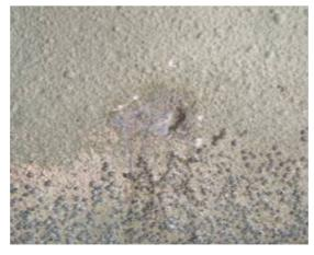
Figure 7: White color which serves as a means by which to evaluate the presence of free chlorides.
