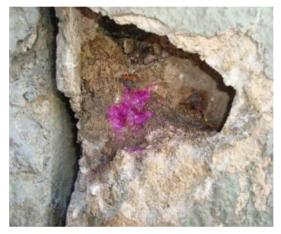
Figure 8: Phenolphthalein solution applied to the newly fractured areas of the structure of the bridge.
