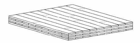
Figure 1.3 – Example of cross-laminated deck plate
