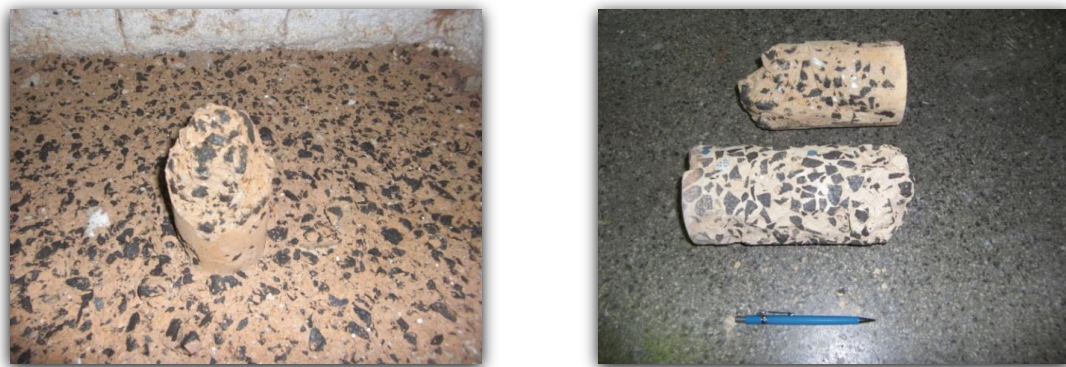
Figure 15. Small cylindrical unreinforced HSC specimens partially disintegrated after fire testing; they had been placed together with the large prototype column.
